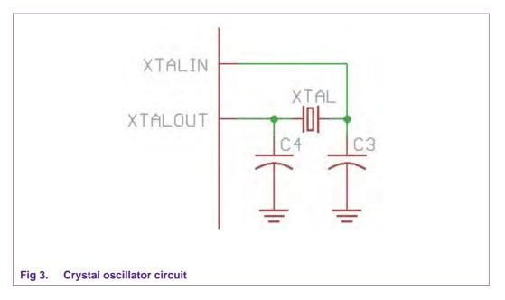
The value of the crystal load capacitors (C3 and C4 in Fig 3) affects the accuracy of the oscillator. The following formula may be used to calculate a parallel resonant crystal's external load capacitors:
