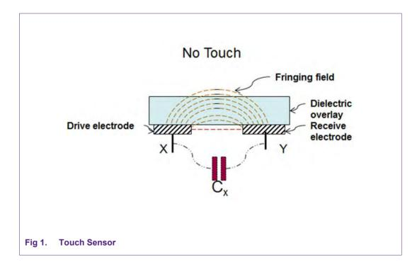
The maximal inter-leaving of X and Y electrodes in T sensor forms a capacitor Cx. When a DC voltage is applied between the X-electrode (driving electrode) and the Y-electrode (receiving electrode) a charge current flows until sensor capacitor Cx is fully charged. The amount of charge flowing into sensor capacitor Cx depends on its capacitance and the applied voltage.
