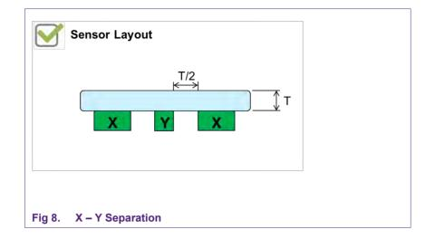
An ideal sensor size is slightly larger than a normal finger. It is recommended to have a sensor size that is slightly larger than the item to be sensed (typically a finger). In general larger keys are more sensitive, but avoid oversized keys as they may have a proximity effect. And undersized keys would result in smaller fringe field in-turn the poor sensitivity. Area of contact from a normal sized finger is about 8mm to 10mm in diameter.
