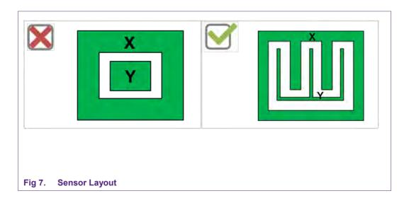
The spacing between X and Y electrodes needs to be at least half the overlay panel thickness. If the overlay panel thickness is T, then the X-Y gap should be at least T/2. There should be no other tracks running below the X-Y gap as this can desensitize the sensor.
