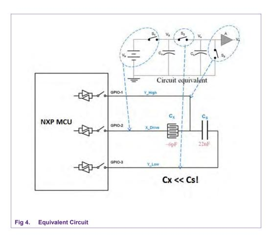
The sensor capacitor Cx forms a part of switched capacitor integrator. The CMOS tri-state drivers connected to the nodes X, Y-H and Y-L are controlled by trains of pulses, resulting in the emulation of integrator switches. The applied pulse sequence causes a repeated charge transport through the sensor capacitor Cx into sample capacitor Cs. With advancing number of integration cycles, an integration voltage Vcs develops across the sample capacitor Cs.
