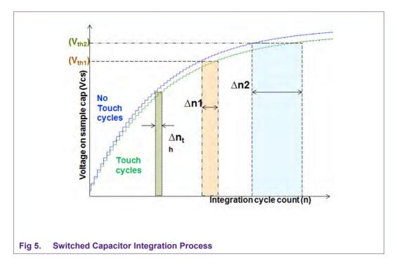
voltage is a measure for the capacitance of sensor capacitor Cx. The integration cycle count performed with no-touch is the reference and forms the basis for Touch detection.
