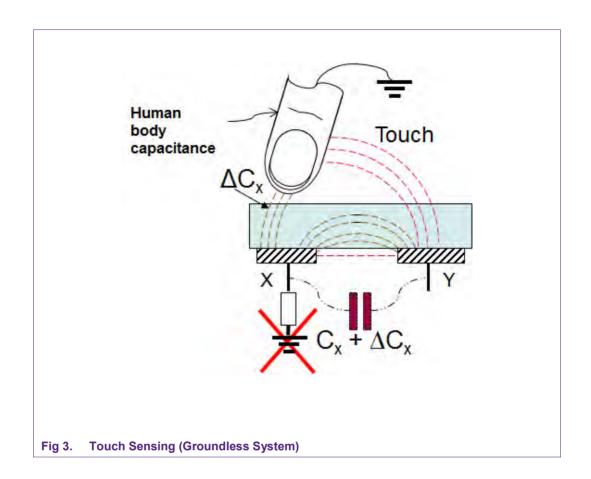
This very small relative change  $(-\Delta Cx \text{ or } + \Delta Cx)$  in the sensor capacitance is detected as a Touch. In addition, there's a lot of post processing involved to increase the robustness, to filter out the noise/jitter, to control the sensitivity, and to compensate for the environmental changes, such as, change in humidity, temperature, or operating voltage.
