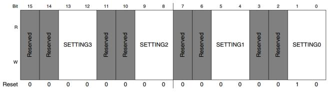
Figure 1. Clock gate registers for peripheral modules
