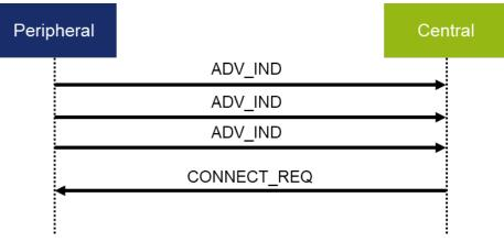
Figure 1. GAP peripheral and central
