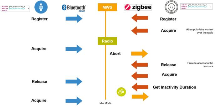
Figure 3. Coexistence of BLE heartrate and Zigbee thermostat
