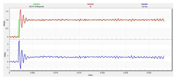
Figure 45. Fast step response of the ld current controller
