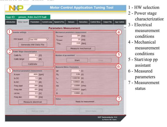
Figure 35. PMSM identification tab
