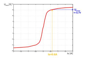
Figure 32. Example power stage characteristic
