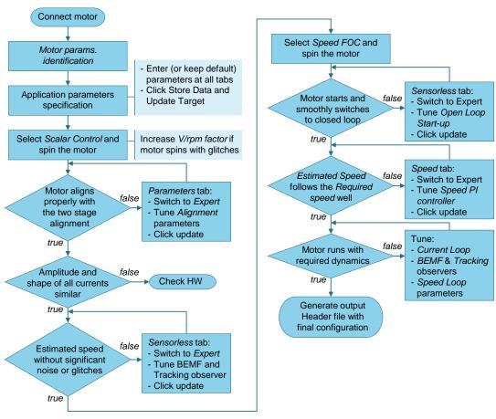
Figure 31. Running a new PMSM
