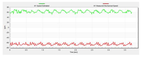
Figure 41. Encoder direction—wrong direction
