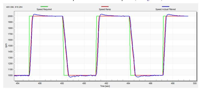
Figure 50. Speed Controller Response—speed loop response with a small overshoot
