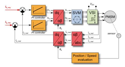
Figure 28. Current (torque) control mode
