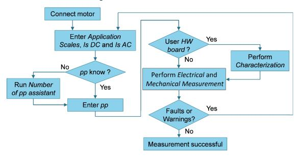
Figure 36. Measurement process diagram
