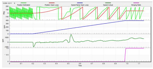
Figure 47. Motor startup
