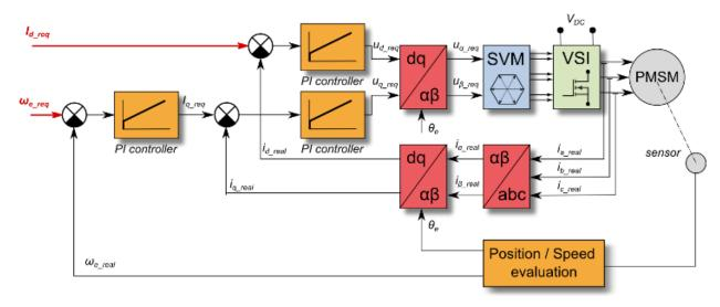
Figure 29. Speed FOC control mode
