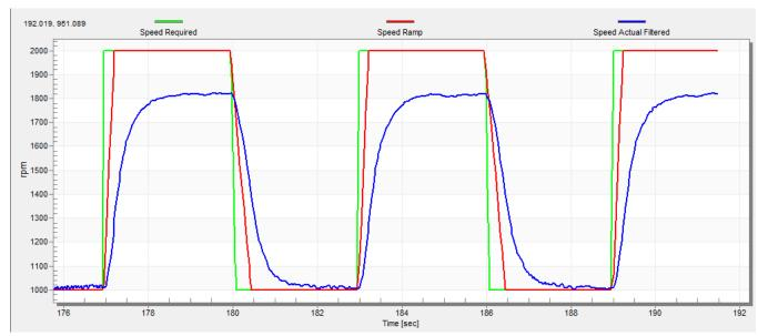
Figure 48. Speed Controller Response—SL\_Ki value is low, Speed Ramp is not achieved
