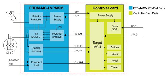
Figure 2. Motor-control development platform block diagram
