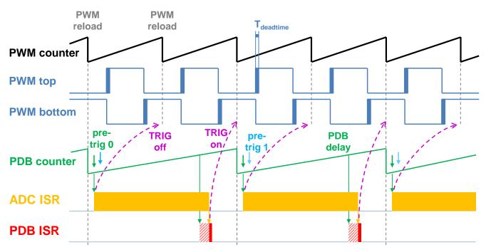
Figure 7. Hardware timing and synchronization on KV31F
