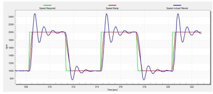
Figure 49. Speed Controller Response—SL\_Kp value is low, Speed Actual Filtered greatly overshoots
