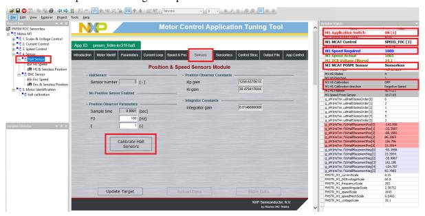
Figure 42. Hall sensors calibration
