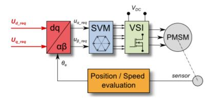
Figure 27. Voltage FOC control mode
