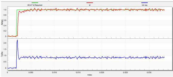
Figure 44. Optimal step response of the ld current controller
