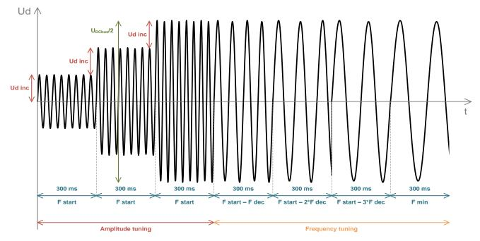
Figure 33. Tuning Ls measuring signal
