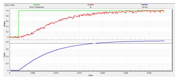
Figure 43. Slow step response of the ld current controller
