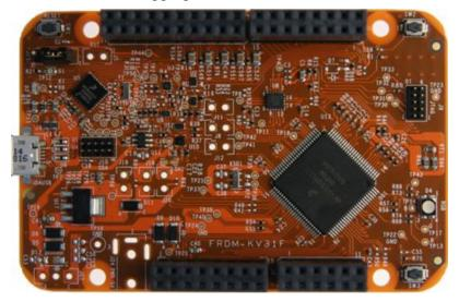
Figure 1. FRDM-KV31F development board
