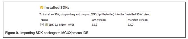
Now, you have downloaded and installed the SDK package for the FRDM-KW36 board.
