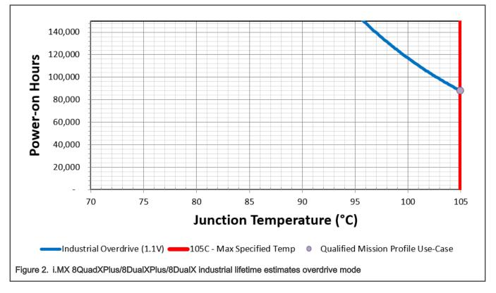
Figure 2 establishes guidelines for estimating PoH as a function of junction temperature. PoH can be read directly from the curves below to determine the necessary trade-offs to the junction temperature at the maximum CPU frequency.
