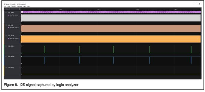
Figure 9 shows that when testing on Window 10, the I2S\_WS is adjusted every 9 seconds. In practice, the frequency of adjusting I2S\_WS is related to the clock of the USB host and the I2S clock of the USB device.
