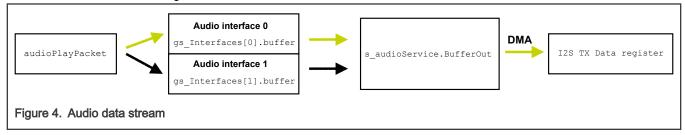
In this example, only one audio interface is implemented and the function of audio mixer is not used, that is, the audio data stream only moves according to the direction of the green arrow of Figure 4.
