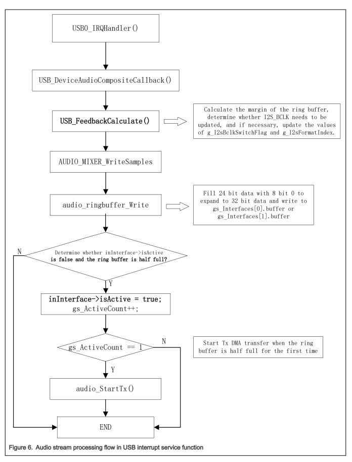
For a full-speed USB audio device, the USB host sends a packet of audio stream data every millisecond, and the packet size is 288 bytes (48 K\*2\*3). It can be seen from Figure 6 that in the USB interrupt service function, the USB\_FeedbackCalculate function is first called to calculate the margin of the ring buffer to determine whether I2S\_BCLK should be updated. If I2S\_BCLK should be updated, update the values of the g\_I2sBclkSwitchFlag and g\_I2sFormatIndex variables.
