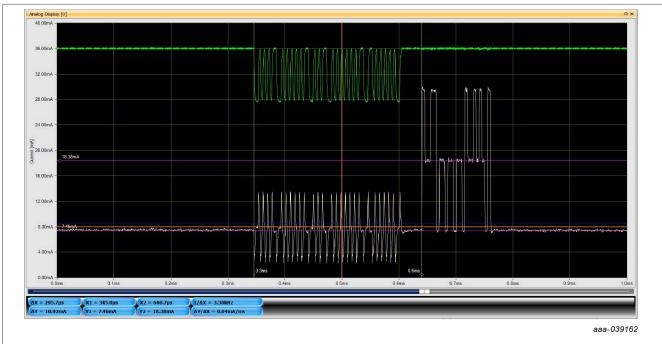
Figure 3. Controller and satellite signals for the global write to the PHYSADDR register
