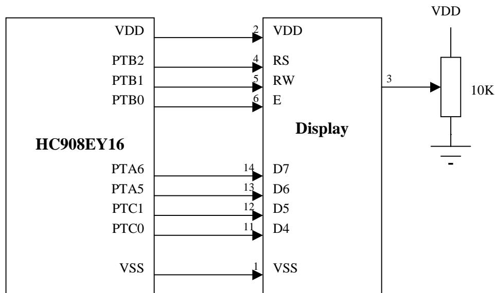
As can be seen from the diagram, only four lines are being used as the data bus between the EY16 & the display. This complicates the software slightly, since any data writes / reads take place over two cycles rather than one. However, this makes the hardware interface much more straightforward, minimising the lines required to drive the display.
