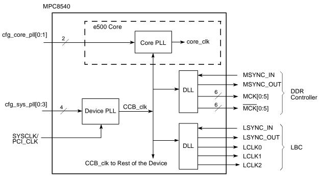
Figure 2. Clock Subsystem Block Diagram
