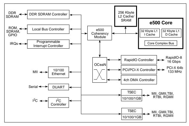
Figure 1. MPC8540 Functional Block Diagram
