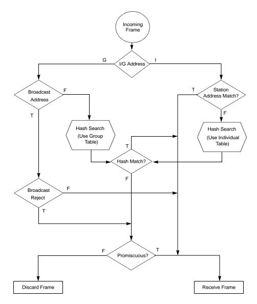
Figure 1. Ethernet Address Recognition Flowchart
