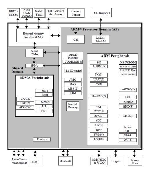
Figure 2. i.MX25 Block Diagram
