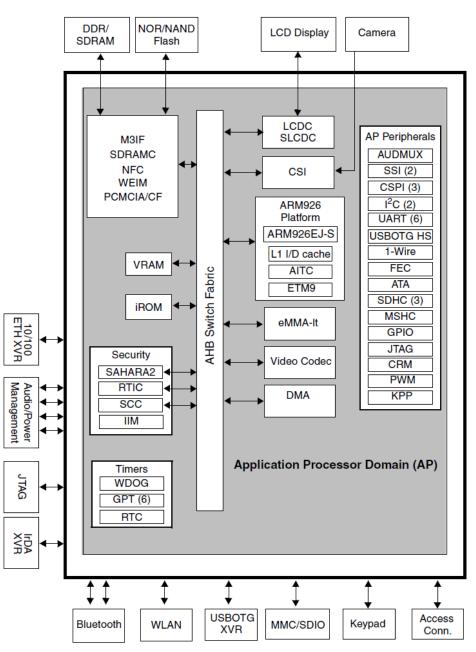
Figure 1. i.MX27 Block Diagram
