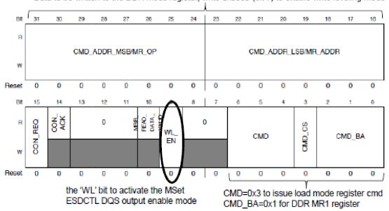
Data to be written to the DDR mode register, write 0x0080 (bit 7) to enable write leveling mode
