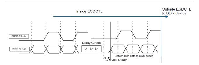
Figure 9. Illustration of Data Being Delayed to Center Align it with DQS
