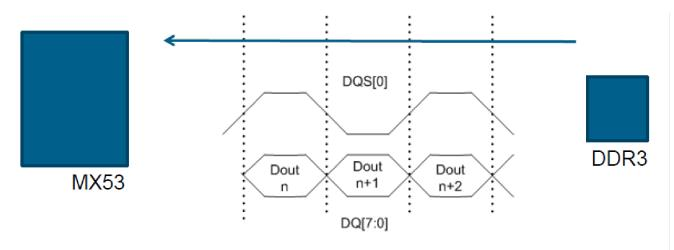
Figure 7. Data read illustration showing edge aligned DQS with DATA
