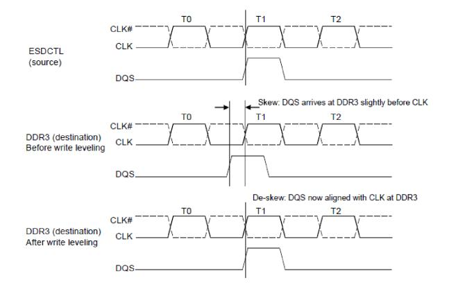
Figure 4. Timing Diagram: Before and After the Write Leveling
