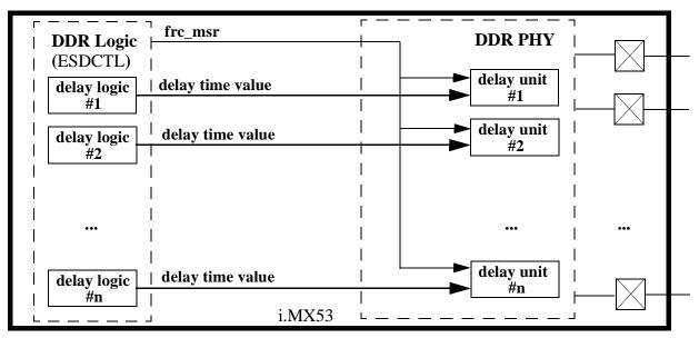
Figure 1. i.MX53 Delay Units Hardware: Functional Diagram
