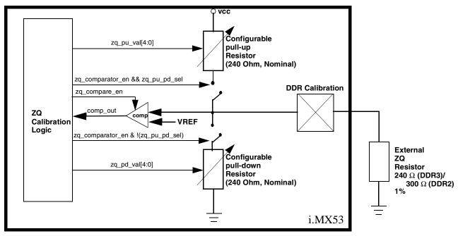
Figure 2. i.MX53 DDR PHY ZQ Calibration Hardware: Functional Diagram
