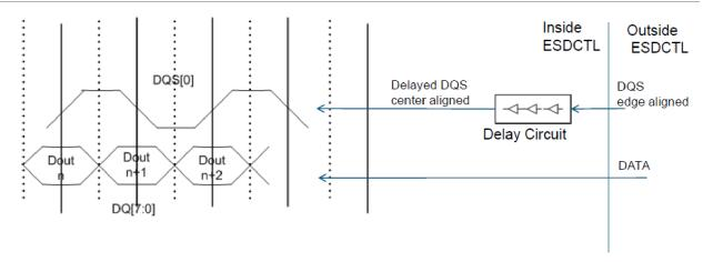
Figure 8. Illustration of DQS Being Delayed to Center Align it with Incoming Read Data
