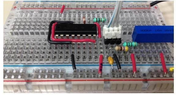
The following figure shows the TIL293D and EE-SX1137 circuitry.
