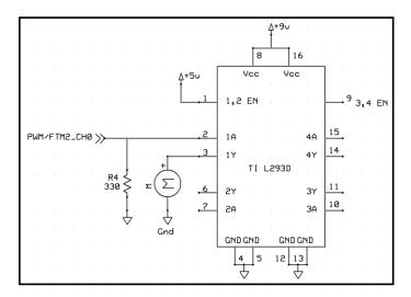
Figure 8 Power stage electrical diagram
