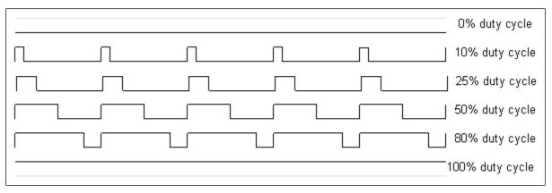
Figure 1 Variable duty cycle signal
