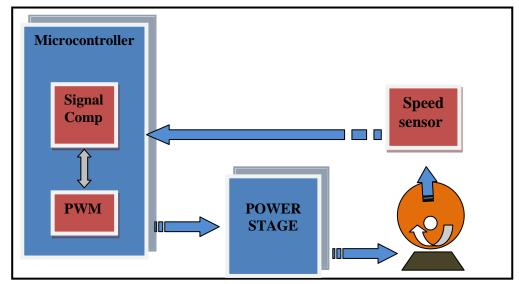
Figure 3 Closed loop PWM motor speed control
