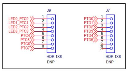
Figure 10 FTM2 and PWT pin assignment
