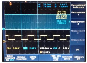
Figure 13 PWM and PWT signals
