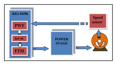
Figure 4 Closed loop PWM motor speed control using the KEx04/06 PWT module
