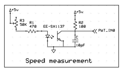
Figure 9 Optical sensor electrical diagram
