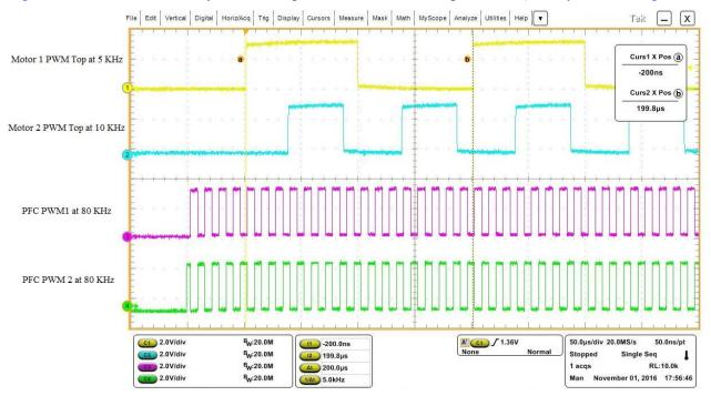
Figure 9. PWMs of Dual motors and PFC at System Start
