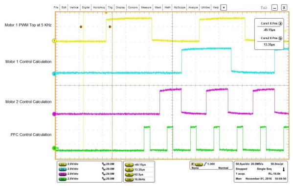
Figure 10. Compressor PWM and ISRs of compressor, fan, and PFC
