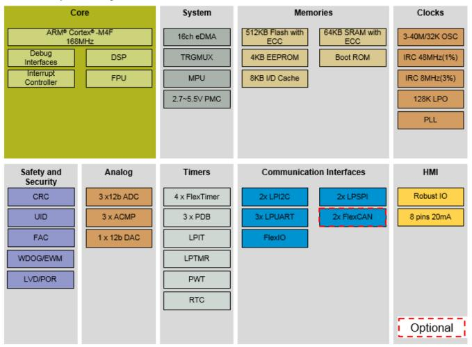
Figure 1. KE1xF MCU block diagram
