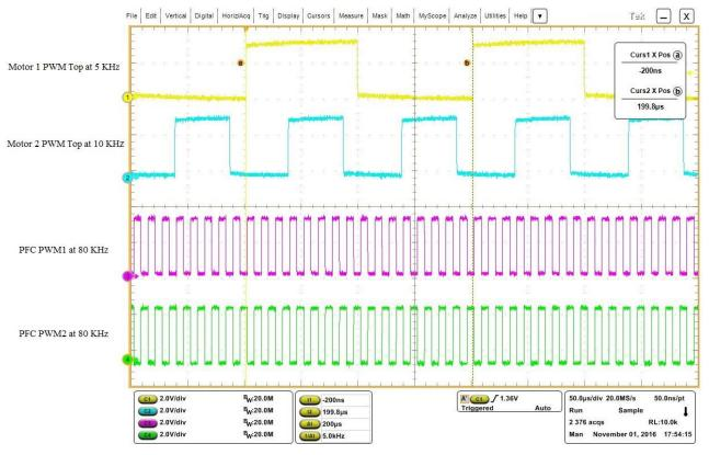
Figure 8. PWMs of Dual motors and PFC
