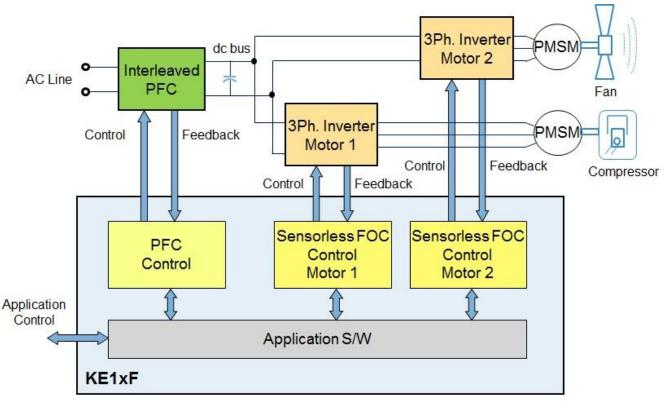
Figure 2. PFC dual motor control concept
