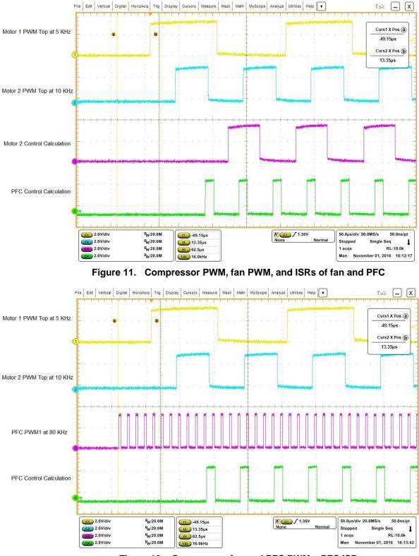
Figure 12. Compressor fan and PFC PWMs, PFC ISR
