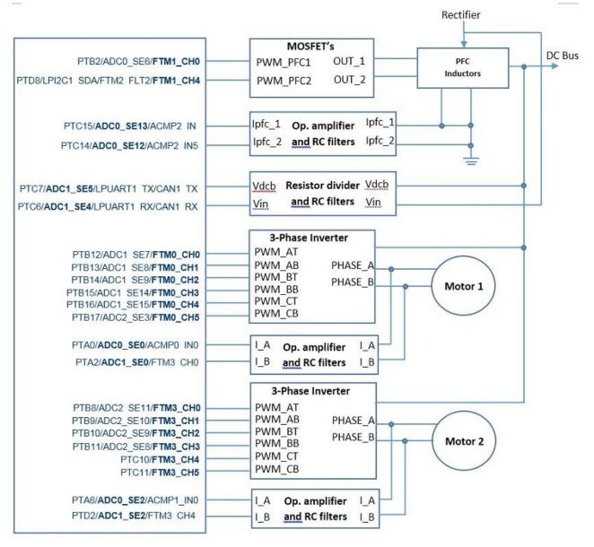
Figure 3. Processor connection to the board circuitry
