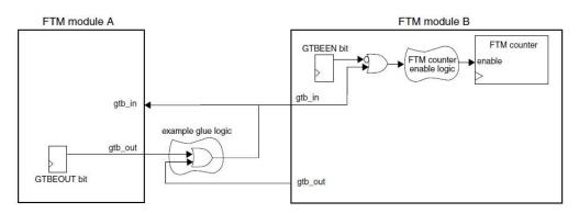
Figure 6. Global time base block diagram
