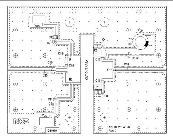
Figure 2. A2T18S261W12NR3 Test Circuit Component Layout
