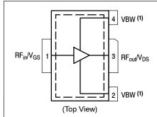
Note: Exposed backside of the package is the source terminal for the transistor.
