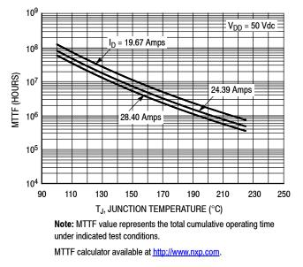
Figure 4. MTTF versus Junction Temperature – Pulse
