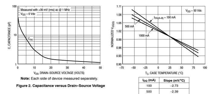
Figure 3. Normalized V<sub>GS</sub> versus Quiescent Current and Case Temperature
