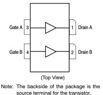
Figure 1. Pin Connections
