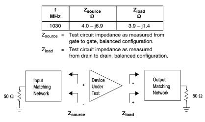
Figure 15. Series Equivalent Source and Load Impedance – 1030 MHz
