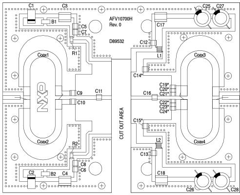
\*C14, C15, C19, C20, C21, C22, C23 and C24 are mounted vertically.
