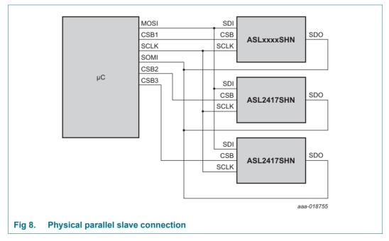
During the SPI data transfer, the identifier byte and the actual content of the addressed registers is returned via the SDO pin. The same happens for pure read accesses. Here the read-only bit must be set to 1. The content of the data bytes that are transmitted to the ASL2417SHN is ignored.
