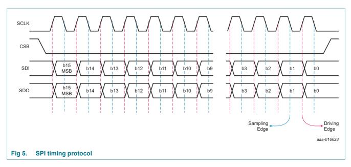
The data bits of the ASL2417SHN are arranged in registers of 1 byte length. Each register is assigned to a 7-bit address. For writing into a register, 2 bytes must be sent to the LED driver. The first byte is an identifier byte that consists of the 7-bit address and one read-only bit. For writing, the read-only bit must be set to "0". The second byte is the data that shall be written into the register. So an SPI access consists of at least 16 bits.
