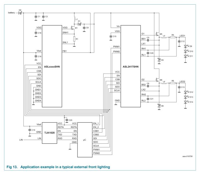
Figure 13 provides an example for the ASL2417SHN in a typical external front lighting application driving 2 independent LED strings.
