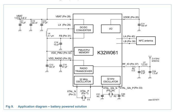
For single-ended antennas or connectors, a balun is not required. However, an external filtering is needed. In receiver, the RFIO pin shows a 50  $\Omega$  impedance and external filtering (R5, C25, L2, C24) is needed in transmission to filter efficiently harmonics. These components are critical and must be placed close to the K32W061 pins and analog ground.
