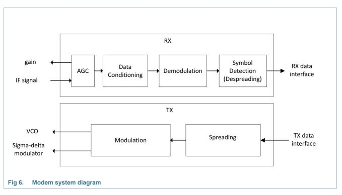
The modem performs all the necessary modulation and spreading functions required for digital transmission and reception of data at 250 kbits/s in the 2.4 GHz radio frequency band in compliance with the IEEE 802.15.4 standard.
