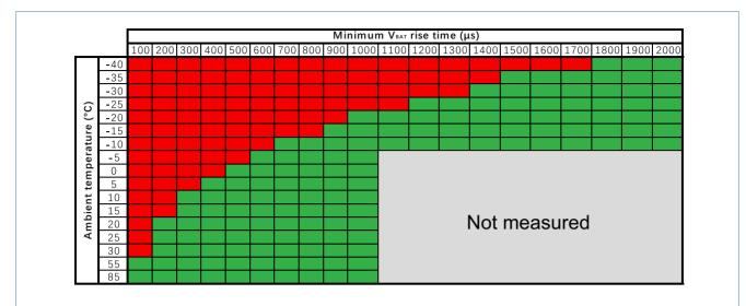
Fig 11. Minimum V<sub>BAT</sub> rise time vs temperature
