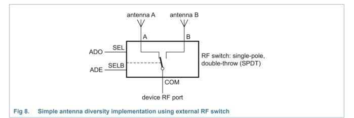
If two DIO pins cannot be spared, one of the signals (ADE or ADO) from the K32W061 can be used and its complement can be generated using an inverter on the PCB.
