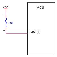
Figure 34. NMI pin biasing
