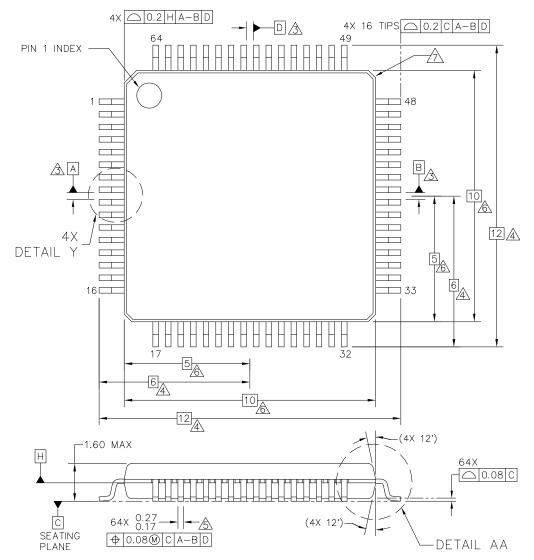
Figure 10. 64-pin LQFP package dimensions 1
