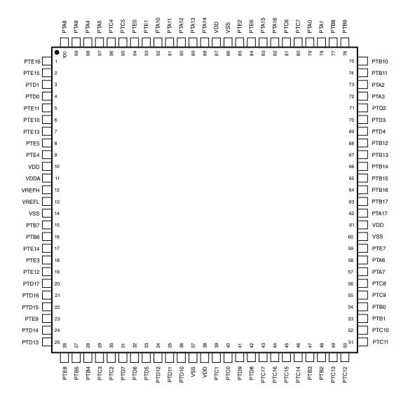
Figure 5. 100 LQFP Pinout Diagram
