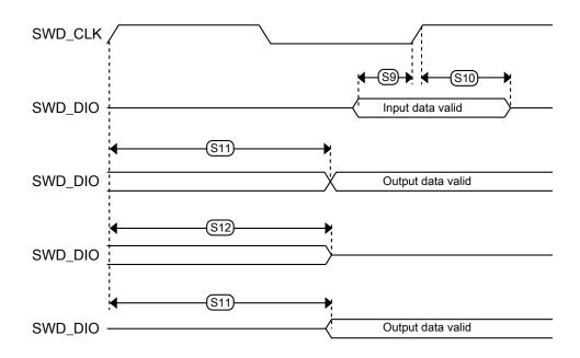
Figure 29. Serial wire data timing
