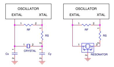
Figure 37. Crystal connection – Diagram 3
