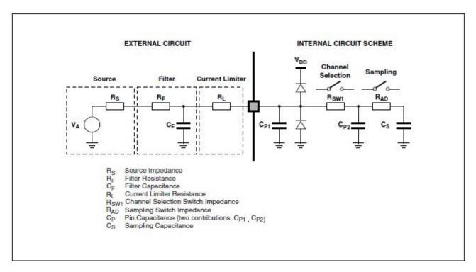
Figure 19. ADC input impedance equivalency diagram
