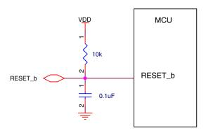
Figure 32. Reset circuit
