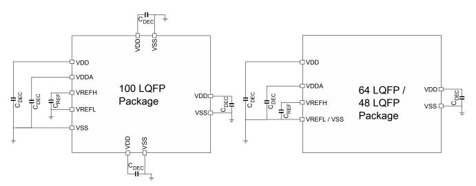
Figure 14. Pinout decoupling
