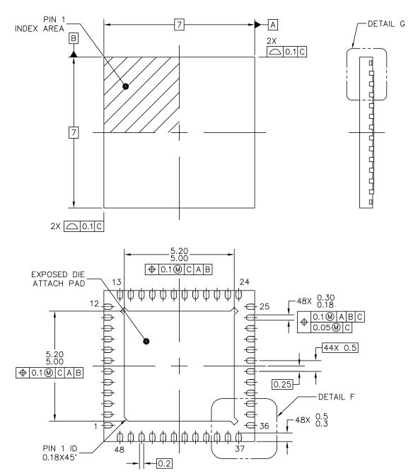
Figure 12. 48-pin QFN package dimension 1
