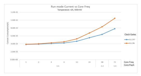
Figure 15. Run mode supply current vs. core frequency
