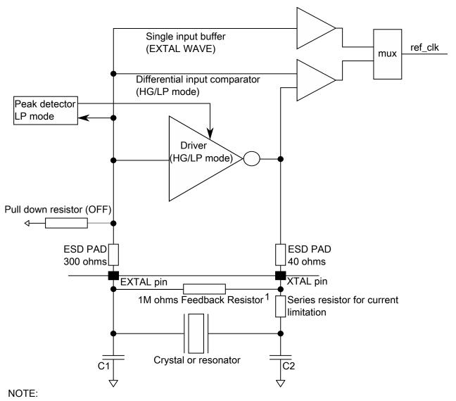
1. 1M Feedback resistor is needed only for HG mode.
