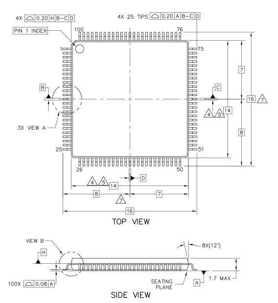
Figure 8. 100-pin LQFP package dimensions 1
