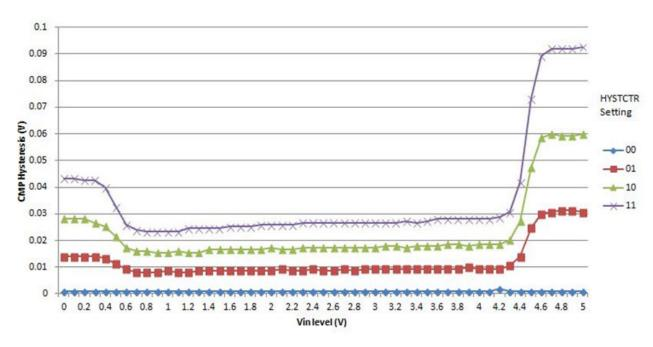
Figure 22. Typical hysteresis vs. Vin level (VDD = 5 V, PMODE = 0)
