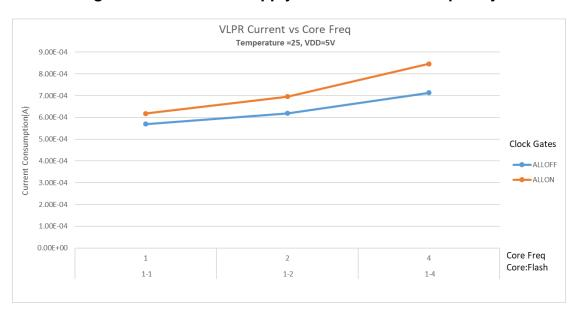
Figure 16. VLPR mode supply current vs. core frequency
