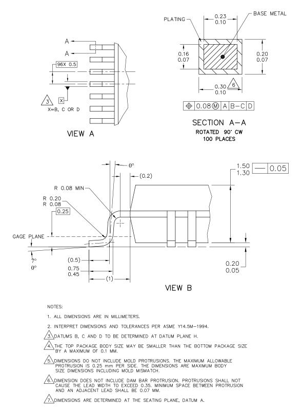
Figure 9. 100-pin LQFP package dimensions 2
