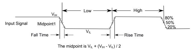
Figure 17. Input signal measurement reference
