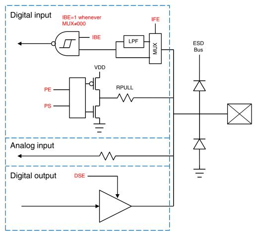
Figure 4. I/O simplified block diagram
