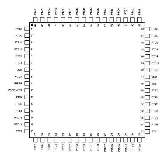
Figure 6. 64 LQFP Pinout Diagram
