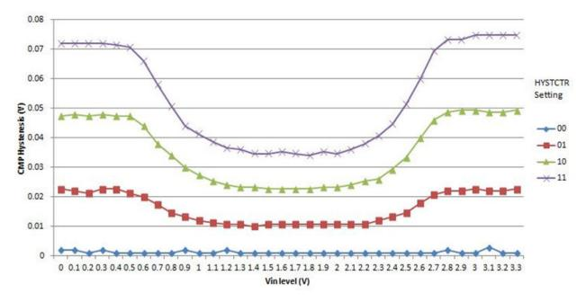
Figure 21. Typical hysteresis vs. Vin level (VDD = 3.3 V, PMODE = 1)
