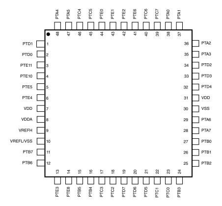
Figure 7. 48 LQFP Pinout Diagram
