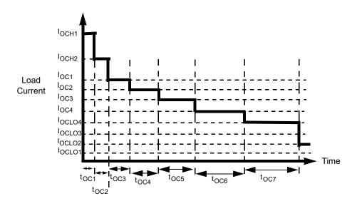
Figure 5. Overcurrent shutdown protection
