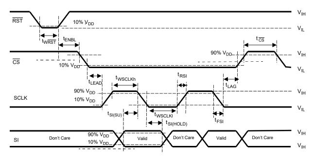
Figure 7. Input timing switching characteristics
