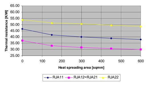
Figure 24. Steady state thermal resistance in dependence on heat spreading area;
