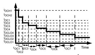
Figure 17. Overcurrent profile depending on Xenon bit
