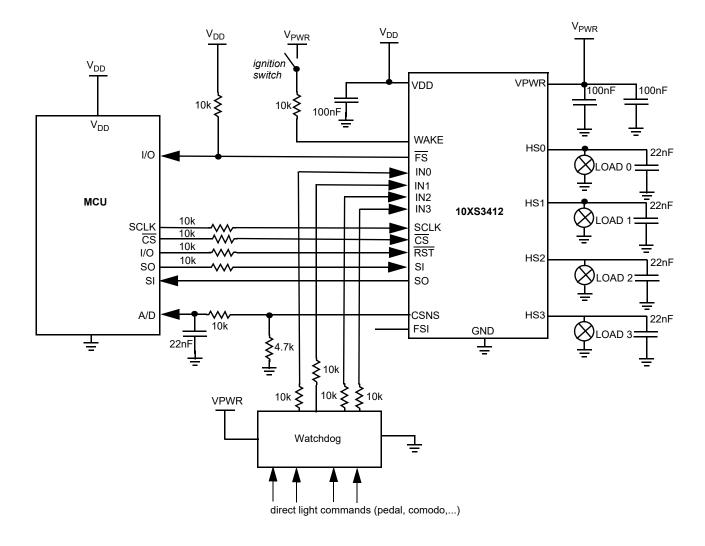
Figure 19. Typical application schematic
