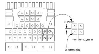
Figure 20. Detail of copper traces under device with thermal vias
