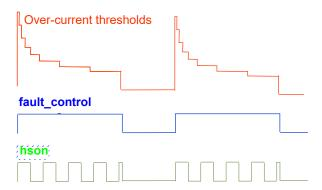
Figure 14. Overcurrent detection profile
