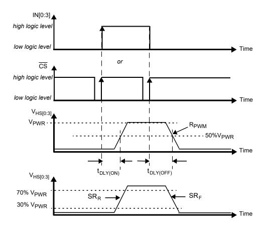
Figure 4. Output slew rate and time delays
