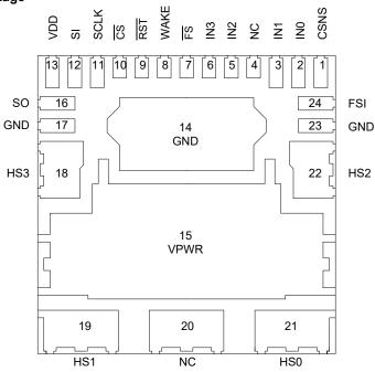
Figure 3. 10XS3412 pin connections
