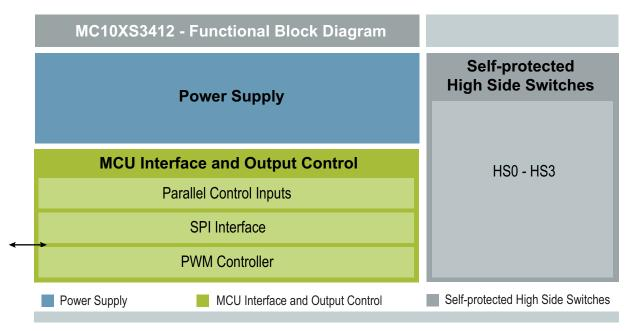
Figure 9. Functional block diagram
