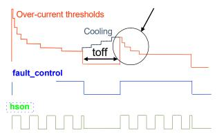
Figure 15. Bulb cooling principle
