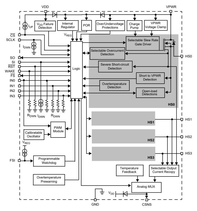
Figure 2. 10XS3412 simplified internal block diagram
