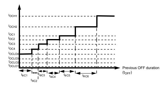
Figure 6. Bulb cooling management
