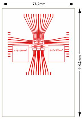
Figure 21. 1s JEDEC thermal test board layout
