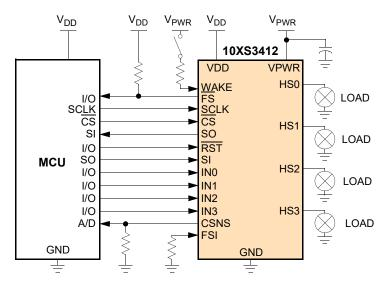
Figure 1. 10XS3412 simplified application diagram
