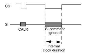
Figure 13. Internal clock calibration diagram
