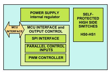
Figure 10. Internal block description
