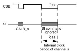
Figure 14. Internal clock calibration
