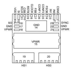
Figure 3. 10XS4200 pin assignments
