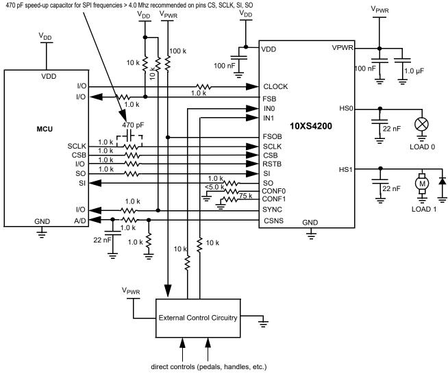
Figure 23. Typical application with two different load types
