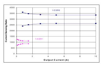
Figure 19. Current sensing ratio versus output current
