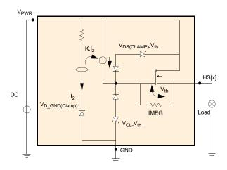
Figure 17. Supply and output voltage protections
