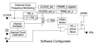
Figure 13. Internal and external clock operation
