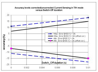
Figure 21. Track and Hold current sense accuracy
