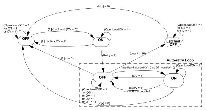
Figure 18. State machine: fault occurrence and auto-retry
