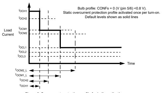
Figure 5. Overcurrent protection profile for bulb applications
