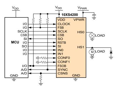
Figure 1. Simplified application diagram
