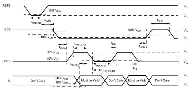
Figure 7. Timing requirements during SPI communication
