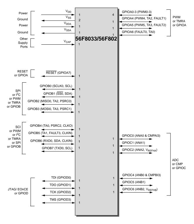
Figure 2-1 56F8033/56F8023 Signals Identified by Functional Group
