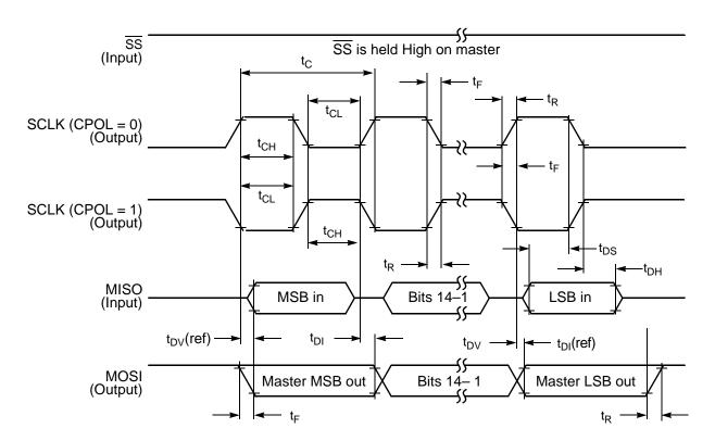
Figure 10-8 SPI Master Timing (CPHA = 1)
