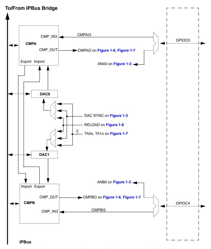
Figure 1-5 56F8033/56F8023 I/O Pin-Out Muxing (Part 3/5)
