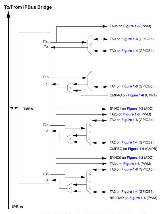
Figure 1-7 56F8033/56F8023 I/O Pin-Out Muxing (Part 5/5)
