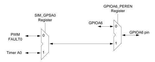
Figure 6-18 Overall Control of Signal Source Using SIM\_GPSnn Control
