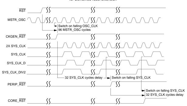
Maximum Delay = 64 OSC\_CLK cycles for POR reset extension and 32 OSC\_CLK cycles for Combined reset extension
