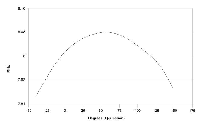
Figure 10-5 Relaxation Oscillator Temperature Variation (Typical) After Trim
