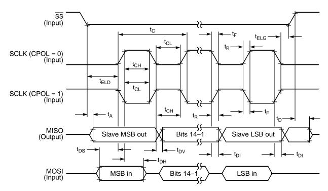
Figure 10-9 SPI Slave Timing (CPHA = 0)
