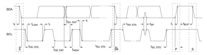
Figure 10-14 Timing Definition for Fast and Standard Mode Devices on the I<sup>2</sup>C Bus
