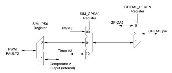
Figure 6-22 Overall Control of Signal Source using SIM\_IPSn Control
