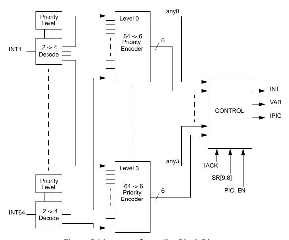
Figure 5-1 Interrupt Controller Block Diagram
