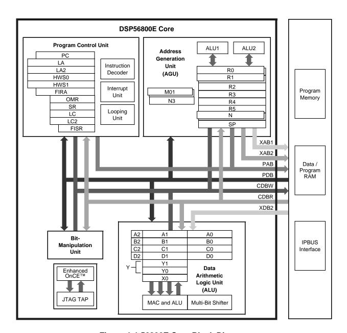
Figure 1-1 56800E Core Block Diagram
