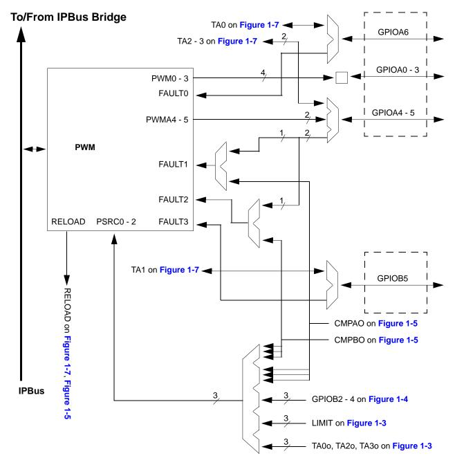
Figure 1-6 56F8033/56F8023 I/O Pin-Out Muxing (Part 4/5)
