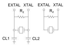
Sample External Crystal Parameters:  $R_z = 750 \text{ K}\Omega$
