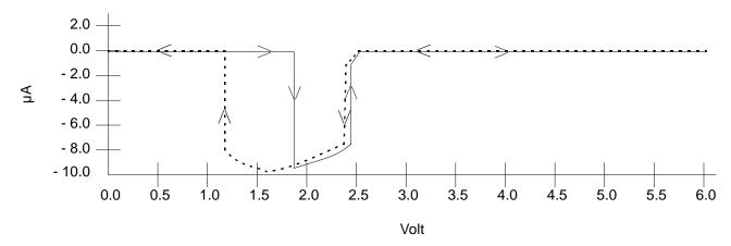
Figure 10-1  $I_{IN}/I_{OZ}$  vs.  $V_{IN}$  (Typical; Pull-Up Disabled)
