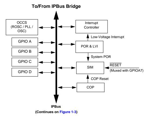
Figure 1-2 Peripheral Subsystem
