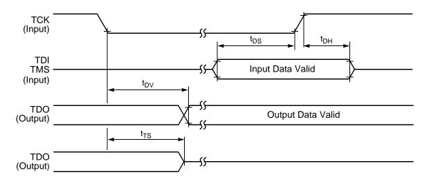
Figure 10-16 Test Access Port Timing Diagram
