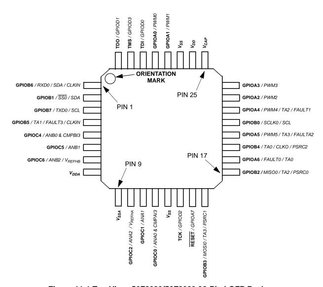
Figure 11-1 Top View, 56F8033/56F8023 32-Pin LQFP Package
