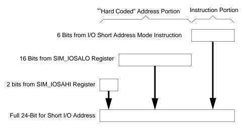
Figure 6-14 I/O Short Address Determination
