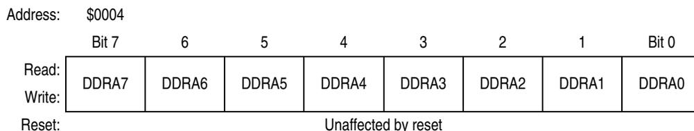
**Figure 27-3. Data Direction Register A (DDRA)**
