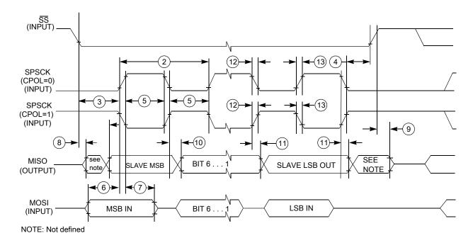
Figure 19. SPI slave mode timing (CPHA = 0)
