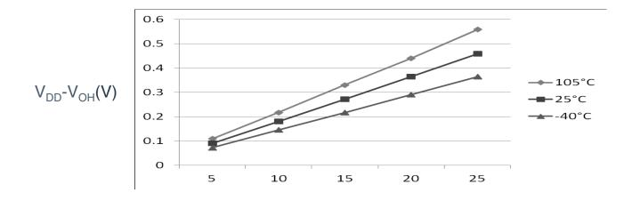
$I_{OH}(mA)$ Figure 3. Typical V<sub>DD</sub>-V<sub>OH</sub> Vs. I<sub>OH</sub> (high drive strength) (V<sub>DD</sub> = 5 V)
