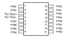
Figure 23. 16-pin TSSOP package
