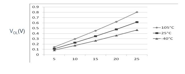
$I_{OL}(mA) \label{eq:IOL}$  Figure 8. Typical V<sub>OL</sub> Vs. I<sub>OL</sub> (high drive strength) (V\_{DD} = 3 V)
