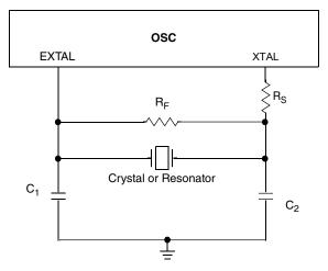
Figure 15. Typical crystal or resonator circuit
