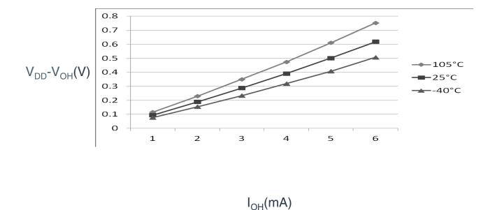
Figure 2. Typical  $V_{DD}$ - $V_{OH}$  Vs. I<sub>OH</sub> (standard drive strength) ( $V_{DD}$  = 3 V)
