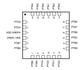
Figure 21. 24-pin QFN package
