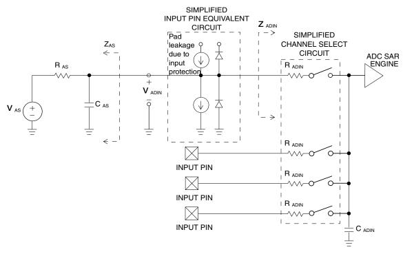
Figure 16. ADC input impedance equivalency diagram
