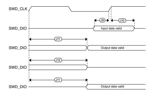
Figure 14. Serial wire data timing
