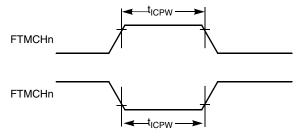
Figure 12. Timer input capture pulse
