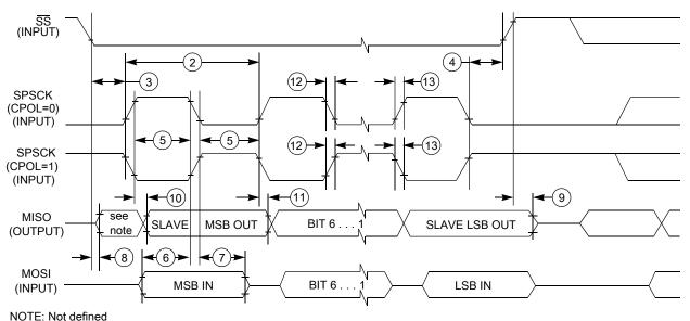
Figure 20. SPI slave mode timing (CPHA=1)
