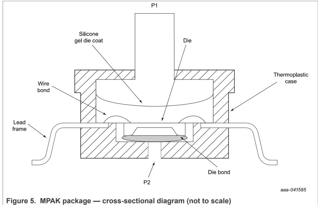
Figure 5. MPAK package — cross-sectional diagram (not to scale)
