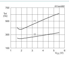
$T_{amb}$  = 25 °C; input overdrive = 100 mV.
