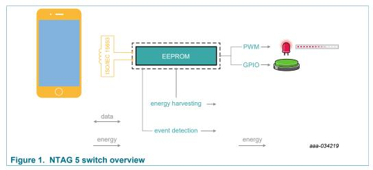
In some lighting and gaming applications, NTAG 5 switch enables simple and cost-effective designs without a microcontroller. It implements multiplexed pins, offering general-purpose I/O (GPIO) and pulse width modulation (PWM) as well as NFC field detection. The characteristics of the PWM or GPIO signal can be configured through the NFC interface. These features can be used to switch on/off and control motor speed or LED brightness.
