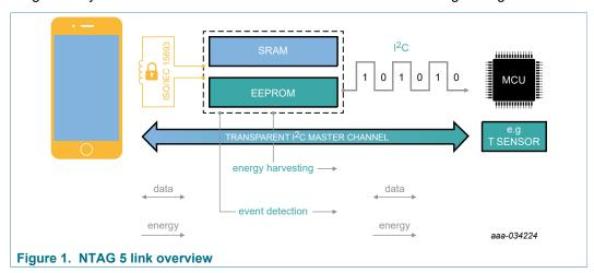
The NTAG 5 link can act as a direct bridge between an NFC-enabled device and any I<sup>2</sup>C slave, such as a sensor or external memory. This is especially useful in environments that require zero-power, single-shot measurements.
