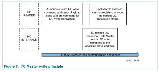
Basic principle for triggering an I<sup>2</sup>C read and getting the response of the connected slave is illustrated in the figure below. Again the NFC reader will get a response immediately, and then polls for the status of the I<sup>2</sup>C transaction (see <u>Table 106</u>). Finally the result can be read from SRAM.
