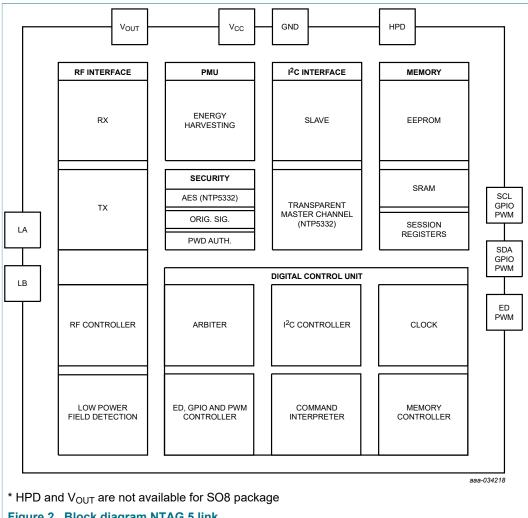
Figure 2. Block diagram NTAG 5 link
