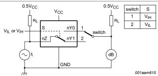
Adjust fi voltage to obtain 0 dBm level at input.
