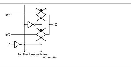
Figure 2. Logic diagram (one switch)
