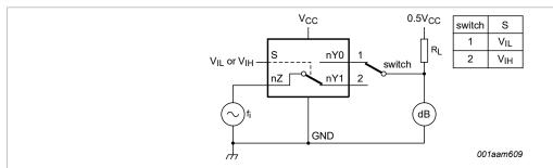
Adjust f<sub>i</sub> voltage to obtain 0 dBm level at output. Increase f<sub>i</sub> frequency until dB meter reads -3 dB.
