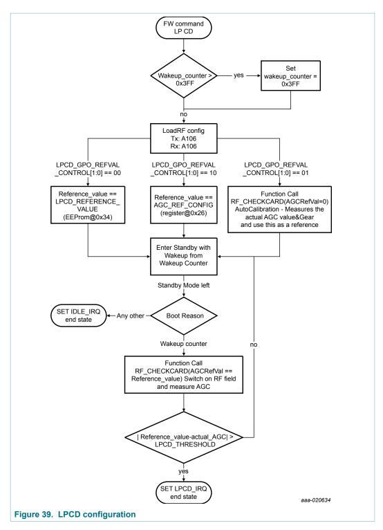
Before entering the LPCD mode, an LPCD reference value needs to be determined. Three options do exist for generating this reference value.
