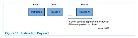
All commands are packed into one SPI Frame. An SPI Frame consists of multiple bytes. No NSS toggles allowed during sending of an SPI frame.
