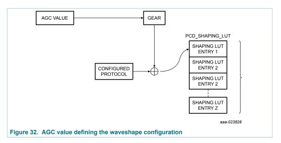
The PN5180 allows measuring periodically the RX voltage. The RX voltage is used as indicator for the actual antenna current. The voltage measurement is done with the help of the AGC. The time interval between two measurements can be configured with the OC\_TIME byte in the EEPROM.
