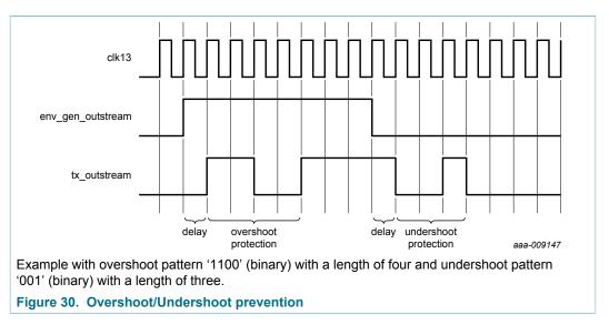
The over- and undershoot protection allows configuring additional signals on the Transmitter output which allows to control the signal shaping of the antenna output.
