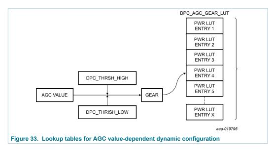
The AGC value is compared to a maximum and minimum threshold value which is stored in EEPROM.
