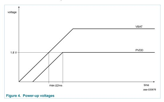
After power-up, the PN5180 is indicating the ability to receive command from a host microcontroller by an IDLE IRQ.
