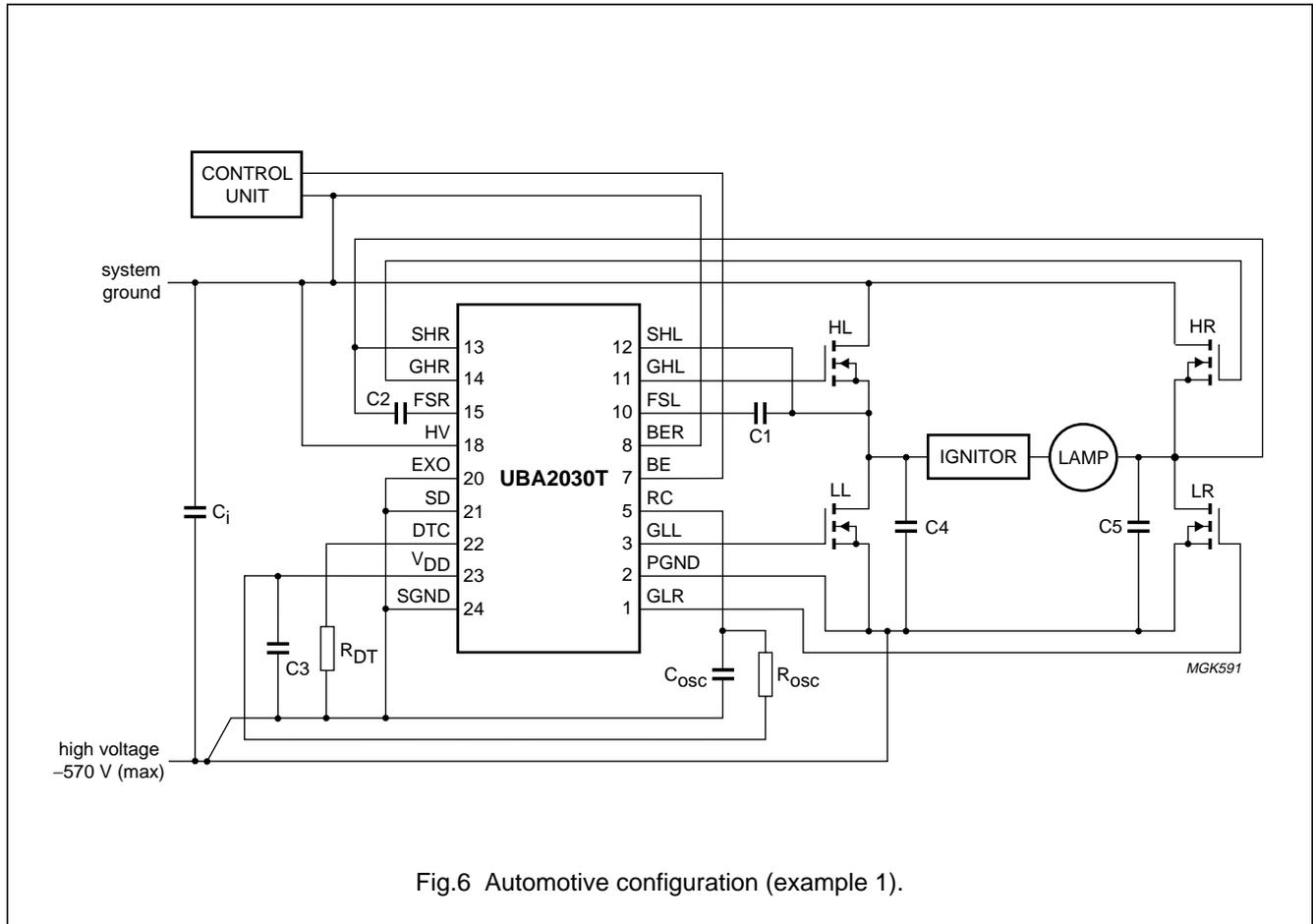
Fig.6 Automotive configuration (example 1).
