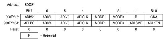
Figure 4. ADC10 Clock Register (ADCLK)
