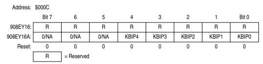
Figure 3. Keyboard Interrupt Polarity Register (KBIPR)
