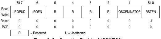
Figure 5. Configuration Register 2 (CONFIG2)
