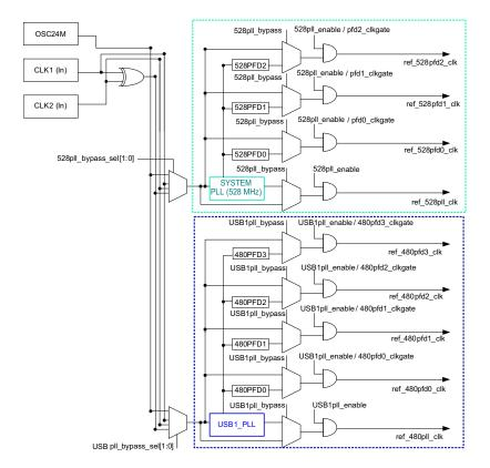
Figure 1. System and USB1 PLL clock generation
