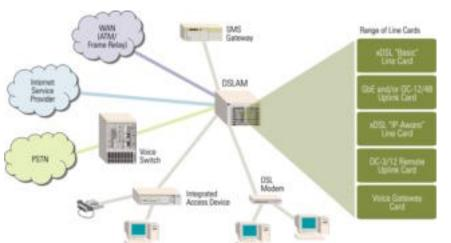
Today's DSL network places demands on a DSLAM system to support high DSL line density for ATM and IP traffic while providing QoS guarantees and other services to individual users
