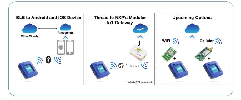
Rapid IoT supports flexible connectivity options for your IoT end node applications. Pre- installed applications combined with a user-friendly interface enable users to quickly select and configure a Cloud connection and create a sensor-to-cloud proof-of-concept
