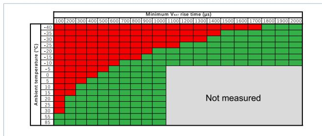
Fig 12. Minimum V<sub>BAT</sub> rise time vs temperature
