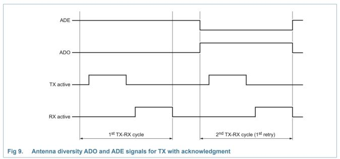
If only one DIO pin can be used, then either ADE or ADO can be connected to the first switch control pin and the same signal inverted on the second pin with an inverter on the PCB.
