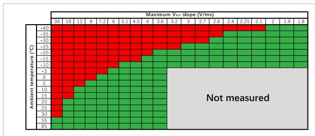
Fig 13. Maximum V<sub>BAT</sub> slope vs temperature
