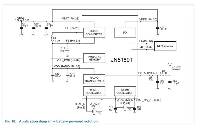
For single-ended antennas or connectors, a balun is not required. However, an external filtering is needed. In receiver, the RFIO pin shows a 50  $\Omega$  impedance and external filtering (R5, C25, L2, C24) is needed in transmission to filter efficiently harmonics. These components are critical and must be placed close to the JN5189 pins and analog ground.
