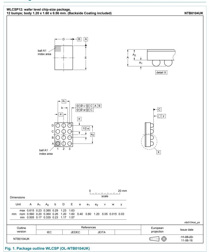
wafer level chip-size package, 12 bumps
