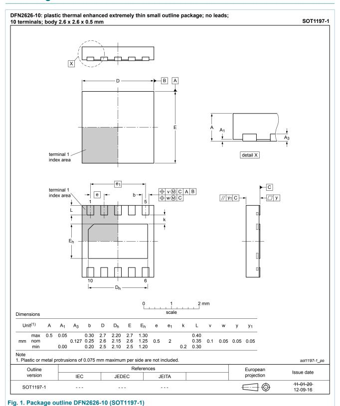
DFN2626-10: plastic thermal enhanced extremely thin small outline package; no leads; 10 terminals
