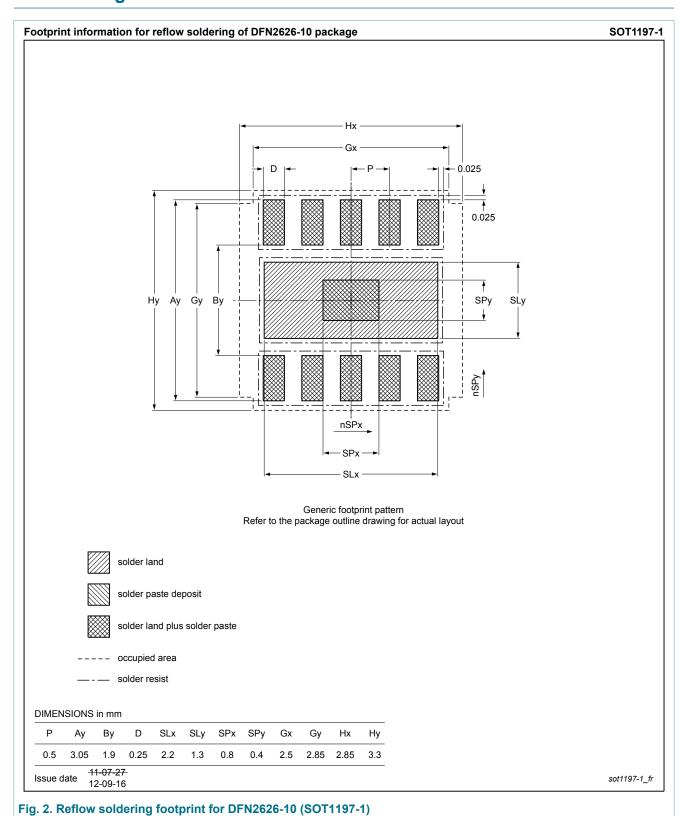
DFN2626-10: plastic thermal enhanced extremely thin small outline package; no leads; 10 terminals
