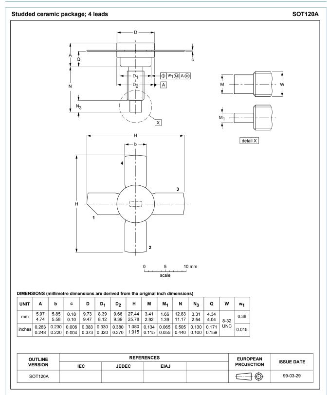
Fig. 1. Package outline CRPM4 (SOT120A)
