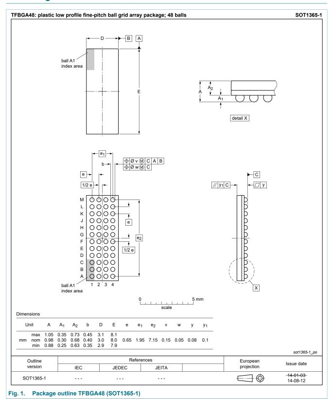
Plastic thin fine-pitch ball grid array package; 48 balls, 0.65 mm pitch, 3 mm x 8 mm x 1.05 mm body
