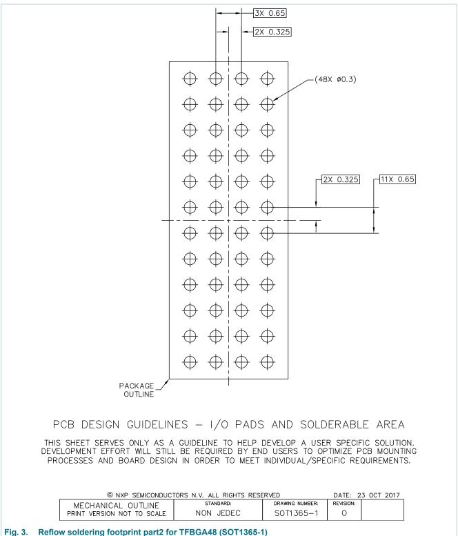
Plastic thin fine-pitch ball grid array package; 48 balls, 0.65 mm pitch, 3 mm x 8 mm x 1.05 mm body
