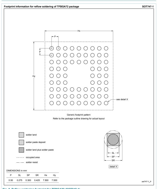
Fig. 2. Reflow soldering footprint for TFBGA72 (SOT747-1)
