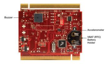
Figure 2: Back side of TWR-K20D72M board
