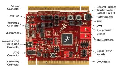
Figure 1: Front side of TWR-K20D72M board
