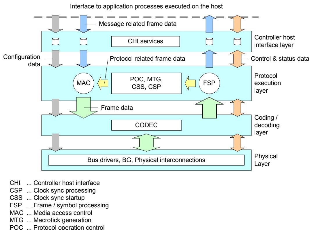
**Figure 2: Conceptual hierarchy of the communications system layers.**
