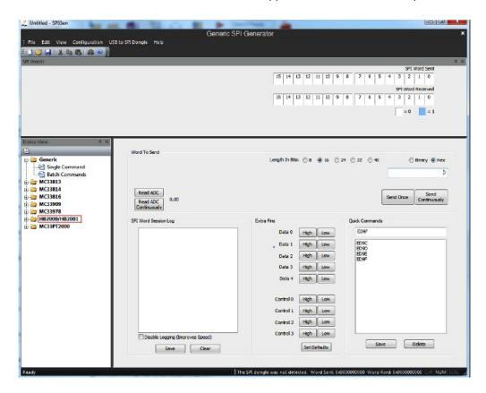
5. To access the HB2000/HB2001 tab in the SPIGen window, expand the HB2000/HB2001 folder in the Device View. Then click **Registers** icon.
