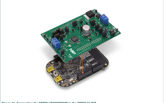
Figure 11. Connecting the FRDM-HB2000FEVM to the FRDM-KL25Z
