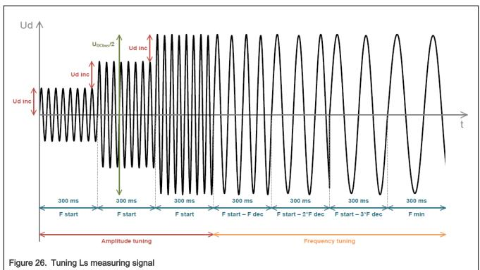
When the tuning process is complete, the sinusoidal measurement signal (with the amplitude and frequency obtained during the tuning process) is applied to the motor. The total impedance of the RL circuit is then calculated from the voltage and current amplitudes and  $L_S$  is calculated from the total impedance of the RL circuit.
