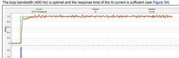
• The loop bandwidth (400 Hz) is optimal and the response time of the ld current is sufficient (see Figure 34).
