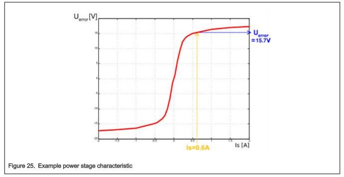
The power stage characterization is necessary only for the user hardware board. When the NXP power stages (TWR, FRDM, or HVP) are used with the application, the characterization process can be omitted. The acquired characterization data is saved into a file, so it is necessary to do it only once for a given hardware.
