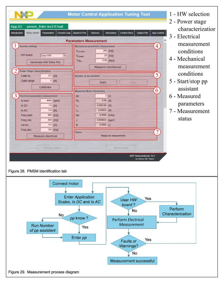
During the measurement, faults and warnings may occur. Do not confuse these faults for the application faults, such as overcurrent, undervoltage, and so on. The list of these faults with their description and possible troubleshooting is shown in Table 8.
