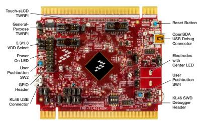
Figure 1: Front side of TWR-KL46Z48M board (TWRPI device not attached)
