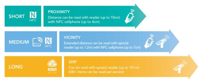
RAIN RFID offers the longest read range, and can read multiple units at once
